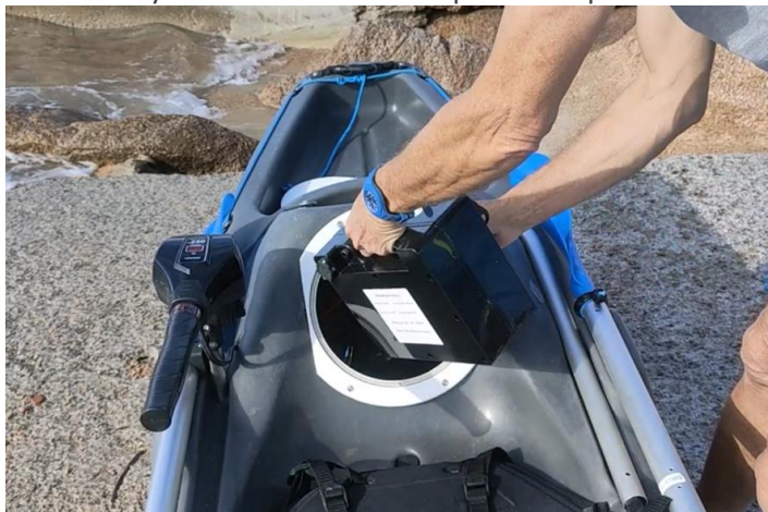
Battery installation in a waterproof compartment
