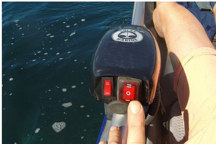
Battery connection, in a waterproof compartment
