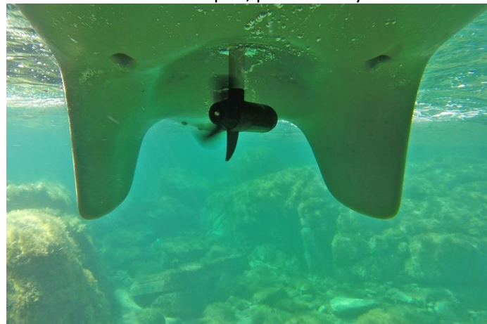
Orientable electric pod, protected by the keels
